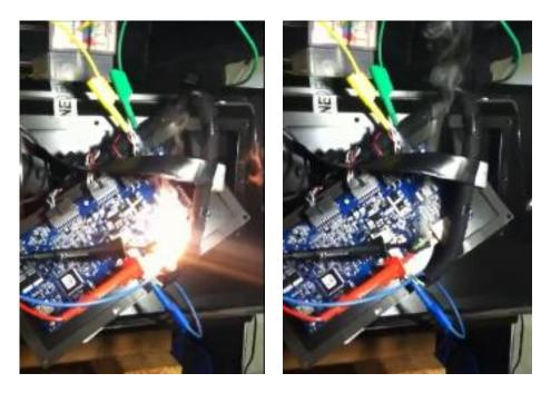
But after the resistor had a chance to cool off it continued to work properly to start up the car, with the exception that it emitted a bright flash of light each time it was energized. There is no telling how long an overheated precharge resistor can go on working properly—or even intermittently—before it finally gives out due to mechanical vibrations or deterioration from repeatedly being energized in a degraded state.
